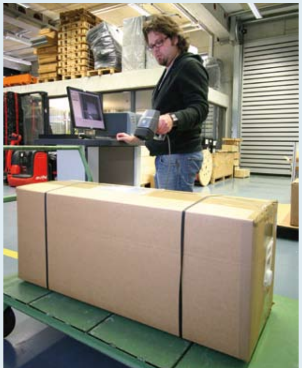
VICAM mobile OCR is connected to a decoding unit by means of cables
