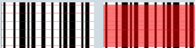
A laser scanner scans at conveyer speed of 2m/s (390fpm) with a sampling rate of 5 scans per 10 millimeters (0,4inch) (above left). A camera scans at conveyer speed of 2m/s (390fpm) with a sampling rate of up to 150 scans per 10 millimeters (0,4inch) (above right).
